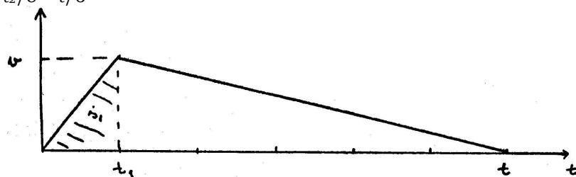
$$s = \frac{v \cdot t}{2} = \frac{v \cdot 6t_1}{2} = 3 \frac{v^2}{a_1} \quad v = \sqrt{\frac{s \cdot a_1}{3}} = \underline{18,71 \text{ m/s}}$$
